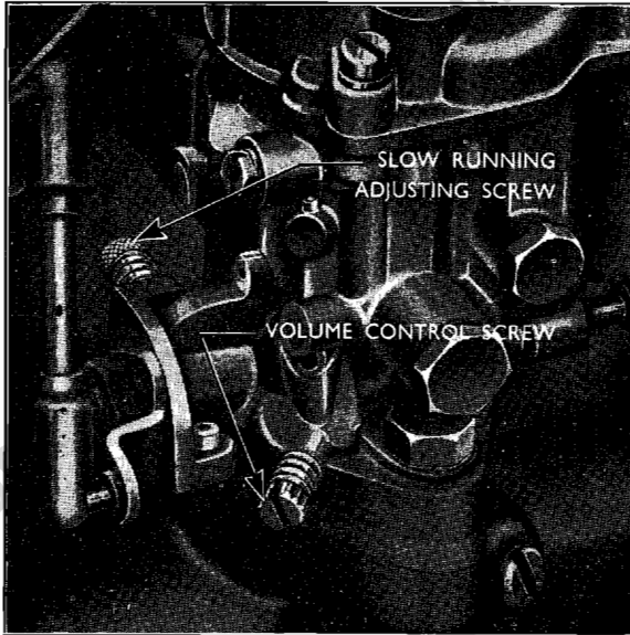
Fig. 11 Slow-Running Adjustments
